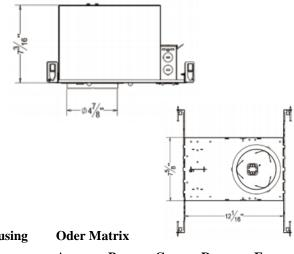
4" Fluorescent IC Airtight Double Wall New Construction Housing
