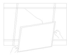
Figure 3, put the panel light on the ceiling position.
