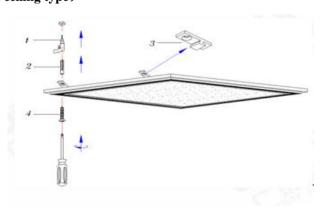
Figure 7, ceiling installation
