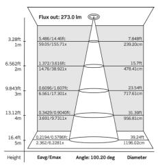
Note: The Curves indicate the illuminated area and the average illumination at a set distance from the LED Down Light.
