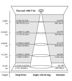
Note: The Curves indicate the illuminated area and the average illumination at a set distance from the LED Down Light.
