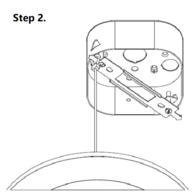
Step 2. Hang one end of the safety rope on the ceiling bracket and hang the disk light.
