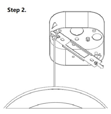
Step 2. Hang one end of the safety rope on the ceiling bracket and hang the disk light.
